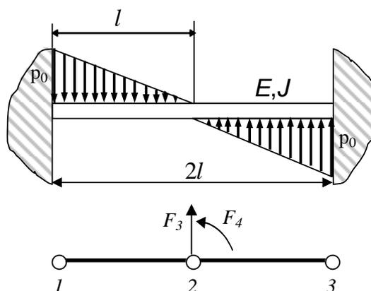
4. Find systems of FEM linear equations before and after considering the constraints.
