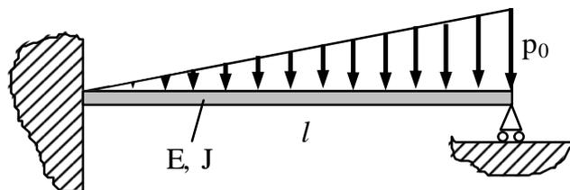
3. Find equivalent nodal forces  $F_3, F_4$ . Write a final system of two linear FEM equations. Find nodal displacements the beam deflection and the bending moment and shear force distributions.
